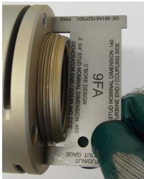
Picture 6C – Use of Stick-Out Gage on Load Coupling or Steam Turbine to Generator Bolted Flange Connection
