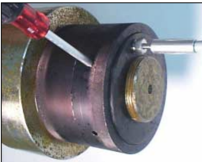
Figure 2 - Hydraulic Tensioner Nut mounted on a flange.
