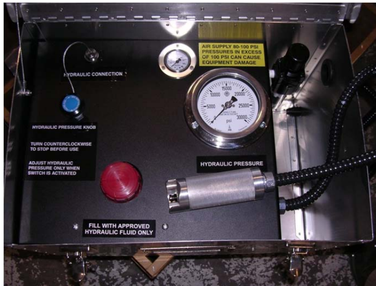
Sample Picture of AP-0532 Hydraulic Pump with hydraulic connection plugged for testing
