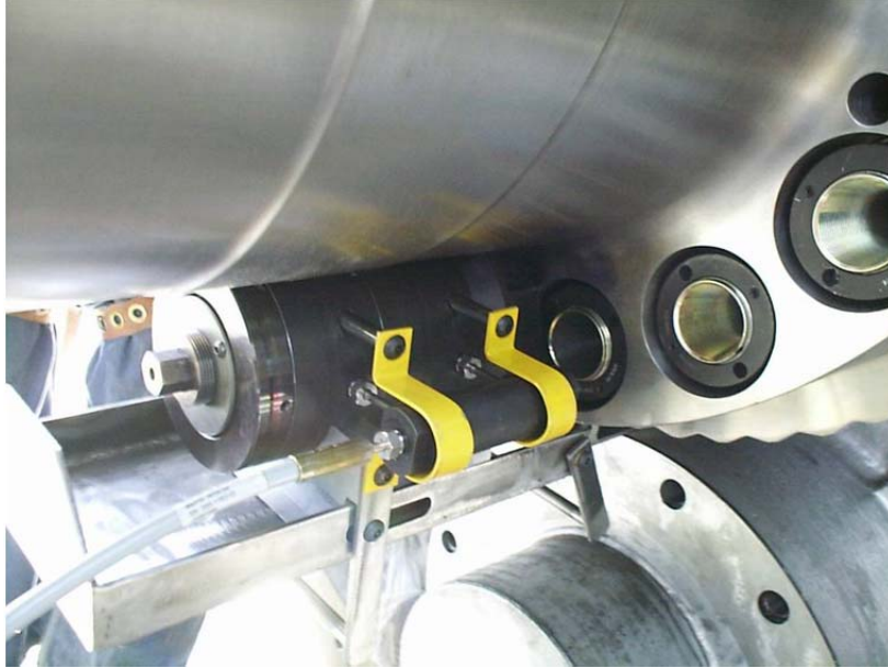
Sample picture showing hose attached to a tensioner
