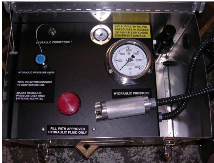
Sample Picture of AP-0532 Hydraulic Pump with hydraulic connection plugged for testing
