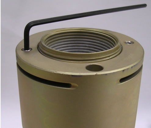
Picture 6 - Loosening of a nut's set screws
