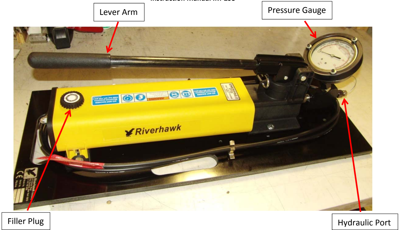
Figure 5 – Sample Picture of MP-6809 Hydraulic Pump with the Hydraulic Port plugged for testing (Right Side)
