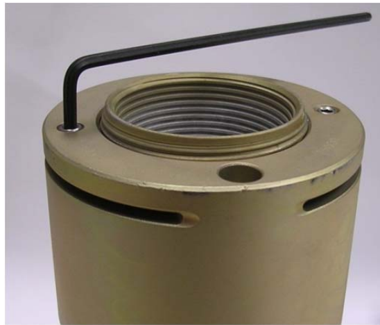
Picture 6 - Loosening of a nut's set screws
