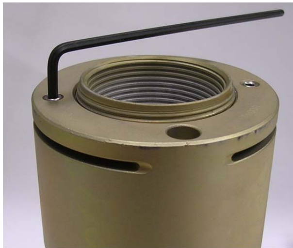
Picture 6 - Loosening of a nut's set screws
