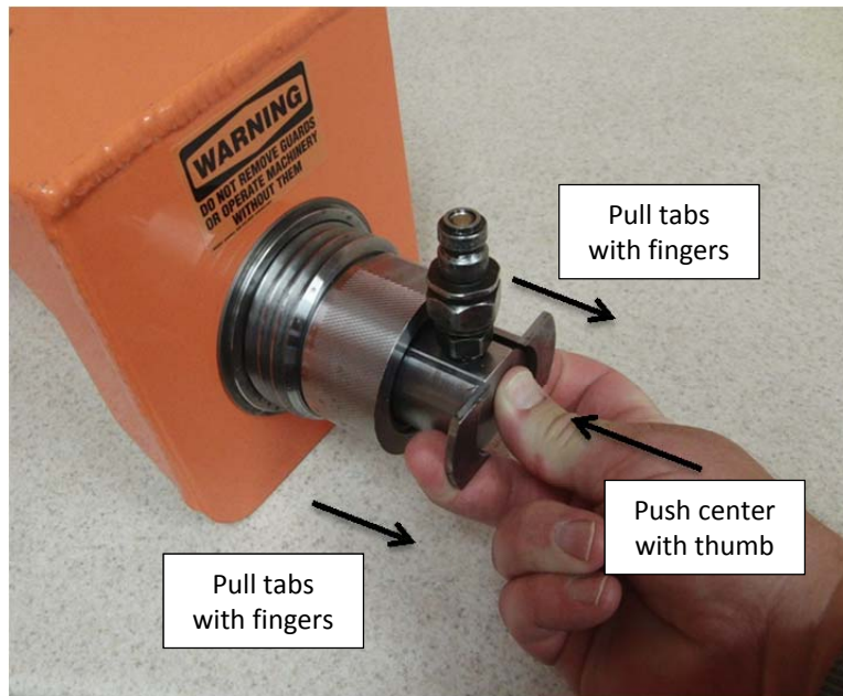
Picture 8E - Activation of the safety interlock
