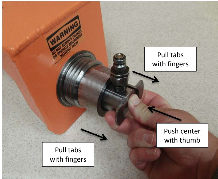
Picture 11B - Activation of the safety interlock
