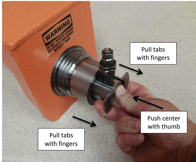
Picture 11B - Activation of the safety interlock
