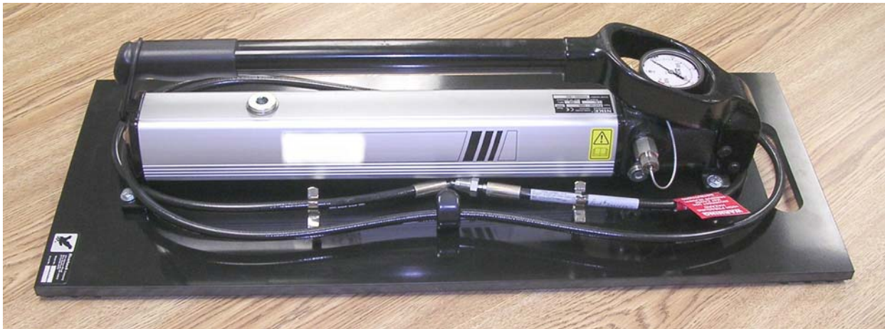
Sample Picture of MP-0130 Hydraulic Pump with hydraulic connection plugged for testing
