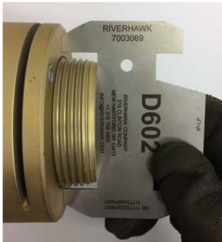
Picture 6E – Use of D602 Stick-Out Gage on the LP/GENERATOR flange connection
