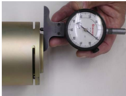
Picture 6G – Use of Drop Gage to measure stick-out
