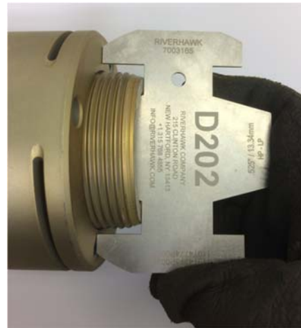
Picture 6E – Use of D202 Stick-Out Gage on the LP/GENERATOR flange connection.
