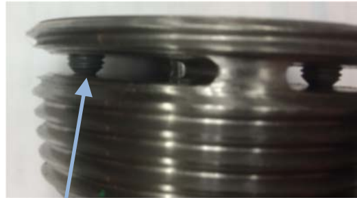
Pressed against Opposite Surface. No Gap
