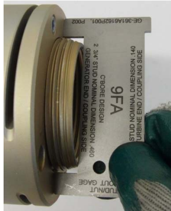
Picture 6C – Use of Stick-Out Gage on Load Coupling to Generator Bolted Flange Connection
