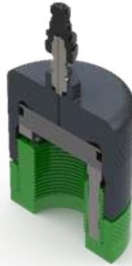
HYDRAULIC ROD TENSIONER (HRT) AND HYDRAULIC ROD NUT (HRN) - HRT SECTION AND ASSEMBLED VIEWS
