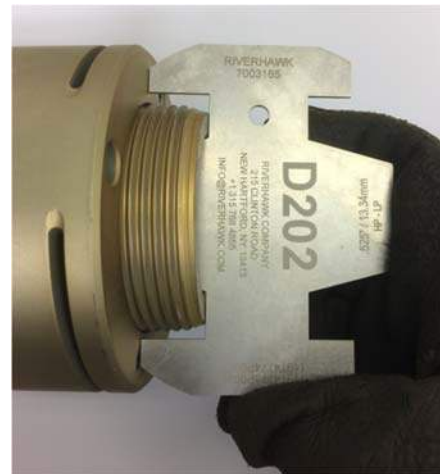
Picture 6F – Use of a D202 Stick-Out Gage on a LP/GENERATOR flange.
