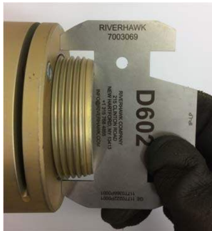
Picture 6E – Use of the D602 Stick-Out Gage on the LP/GENERATOR flange.
