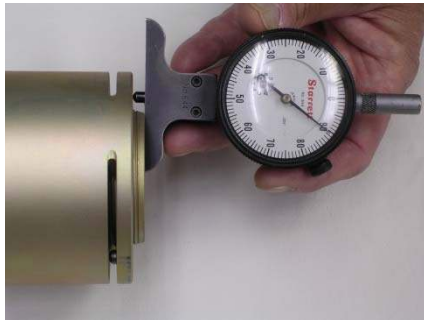
Picture 6H – Use of Drop Gage to measure stick-out
